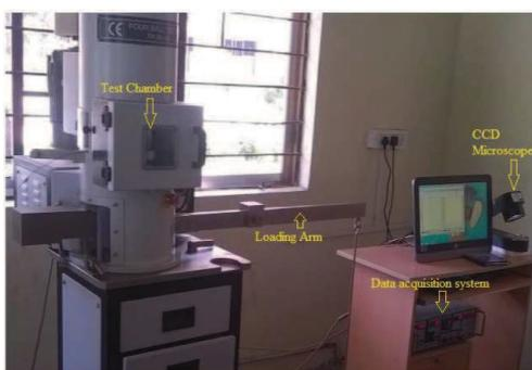
Fig -1: Four ball tribometer
